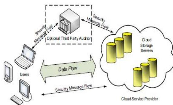
Figure 1: Cloud Data Storage Architecture
